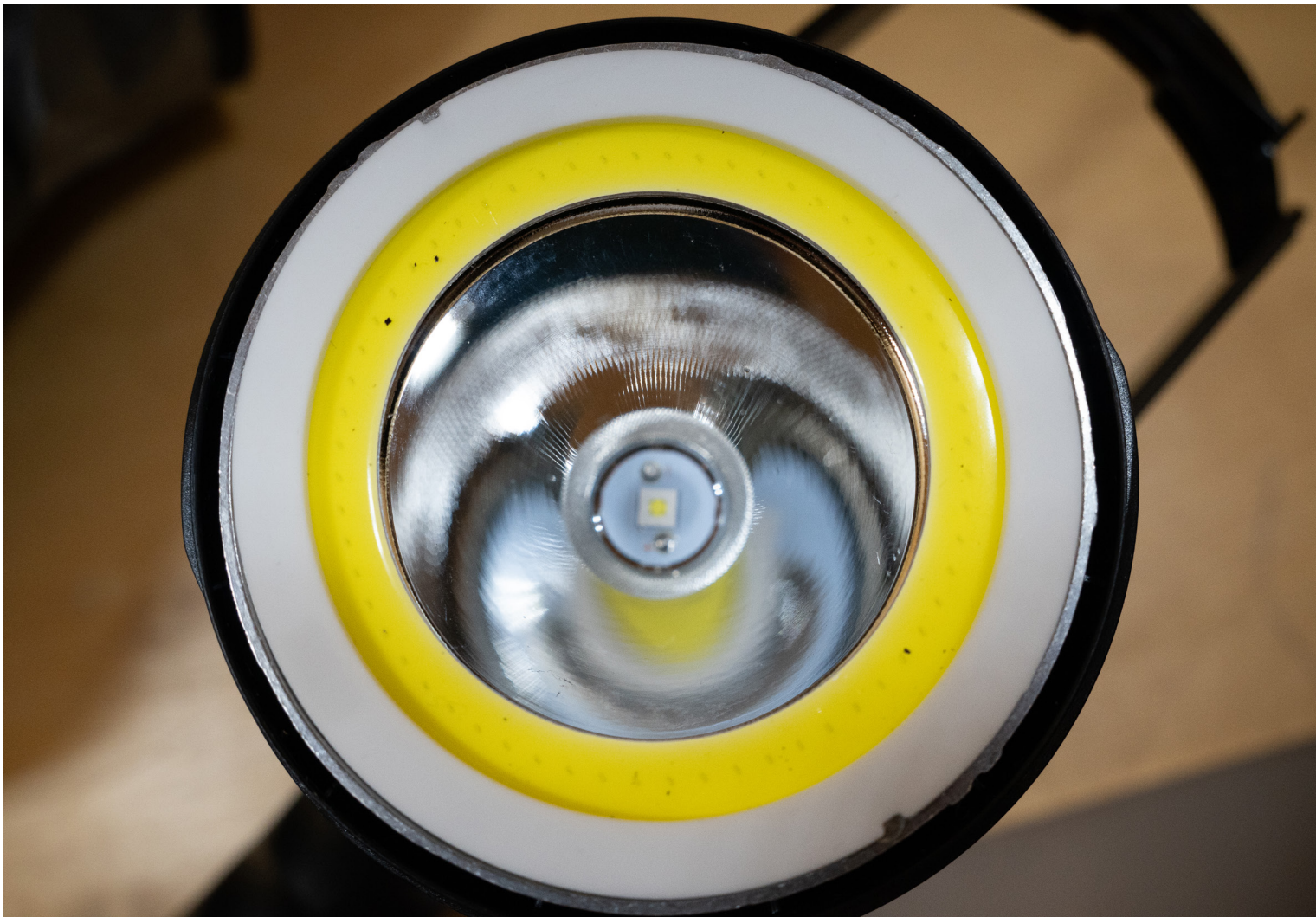
The aim of the cone was simple; to make the beam wider, without dimming. The device itself was attached to a reflective cone to produce a wider aperture to help shine brighter.
