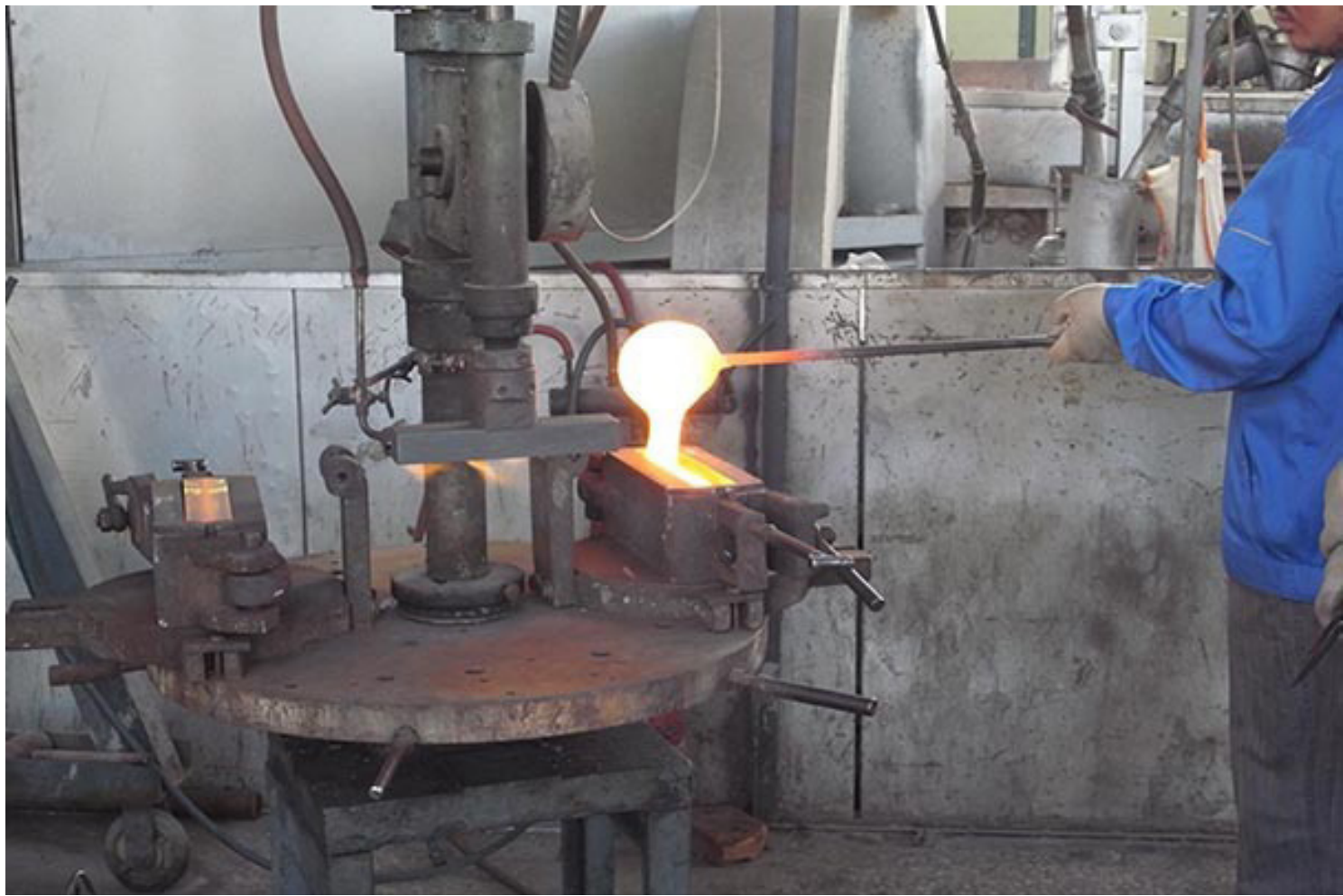
Borosilicate glass, crucial for its optical properties, begins as a molten material in the casting process.
